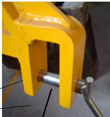
The Meliorator has an ordinary Type 2 three-point-linkage, which implicates that the bolts have the diameter of 28 mm
