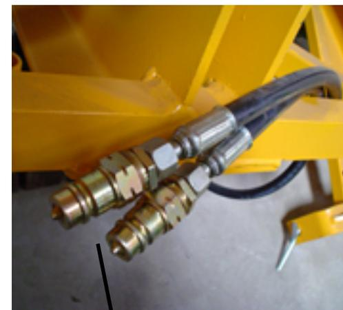
These two hoses are the connectors to the double-acting cylinder on the Meliorator. They are common 1/2" (half inch) hydraulic clutches (male plugs). The tractors must have the corresponding double-acting hydraulic control with the corresponding hydraulic clutches (female connector). It is essential that these demands be met properly. Without this double-acting hydraulic system it is impossible to use the Meliorator at all.
